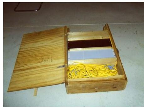
The section with the lights swings out and up then is secured with wing-nuts. A crosspiece at the bottom rotates 90-degrees and is tightened with a wing nut for stability – then close the cover to hide the wires. It's about 5-feet tall.
